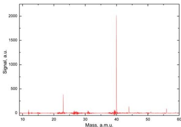
**Figure 2** RIMS spectra of Ca from glass standard reference material.  $^{40}\text{Ca}$  peak is clearly seen. REMPI with one tunable Ti-sapphire laser: fundamental radiation with 719.568 nm (1.72 eV photon) is used for the ionization step, and the 3<sup>rd</sup> harmonic radiation with 239.856 nm (5.17 eV photon) is used for resonant excitation from groundstate to intermediate state.
