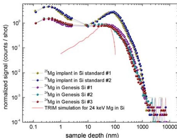
**Figure 1** Depth profiles of SW Mg in Si compared to the Mg implant standard reference material
