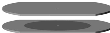
Figure 1. Design of planar resistive electrode ion trap, consisting of two ceramic plates, each coated with metal rings (not visible) and germanium (dark gray).
