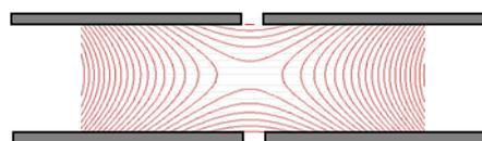
Figure 2. Electric field lines on the planar resistive electrode ion trap.
