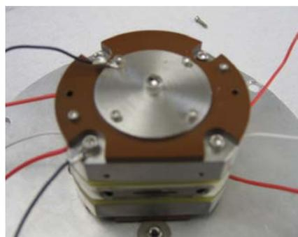
Figure 3. Prototype model of planar resistive electrode ion trap (toroidal geometry), including mounts and voltage divider.
