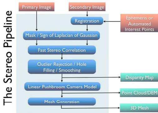
Figure 1. ASP processing flow diagram.
