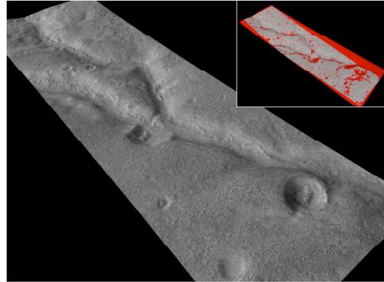
Figure 2. This 3D terrain model was generated from MOC-NA images. The inset in the upper right shows areas of interpolated data where the stereo correlation failed to find a match.
