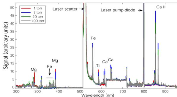
**Figure 3:** Full spectrum of micro-LIBS on hematite [8].
