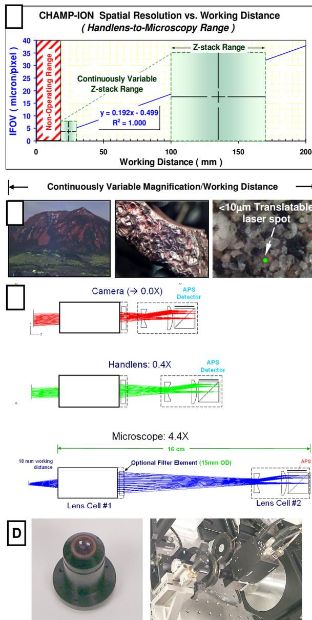
**Figure 1.** A) Raman/CHAMP instrument pixel resolution vs. working distance. B) Images from earlier MIDP version of CHAMP instrument continuously variable magnification with simulated scan-able object-plane Raman laser spot (exaggerated in size for clarity) at peak magnification; C) Instrument optical layout and lens cell variable magnification/working distance actuation; D) Fabricated Lens Cells integrated into brass-board test setup.
