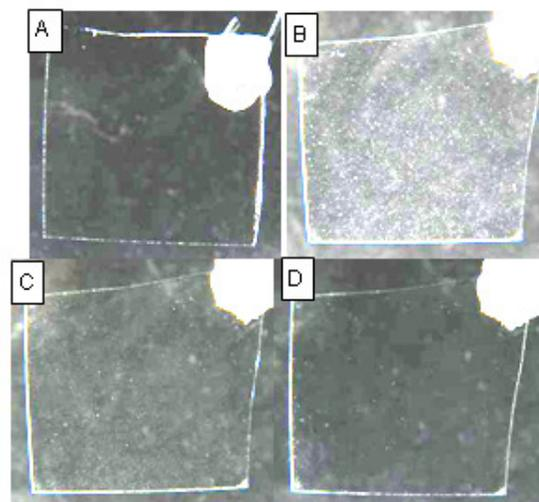
**Figure 4.** micro-LIBS condensate deposit on window before and after laser shots at 100  $\mu J$ , working distance of 15mm, with F/#4 CHAMP-like distal beam. A) Typical slide before image, B) slide after 17,700 laser shots, C) used window after 3 sec air blast and D) following 3 wipes with lens brush [9].
