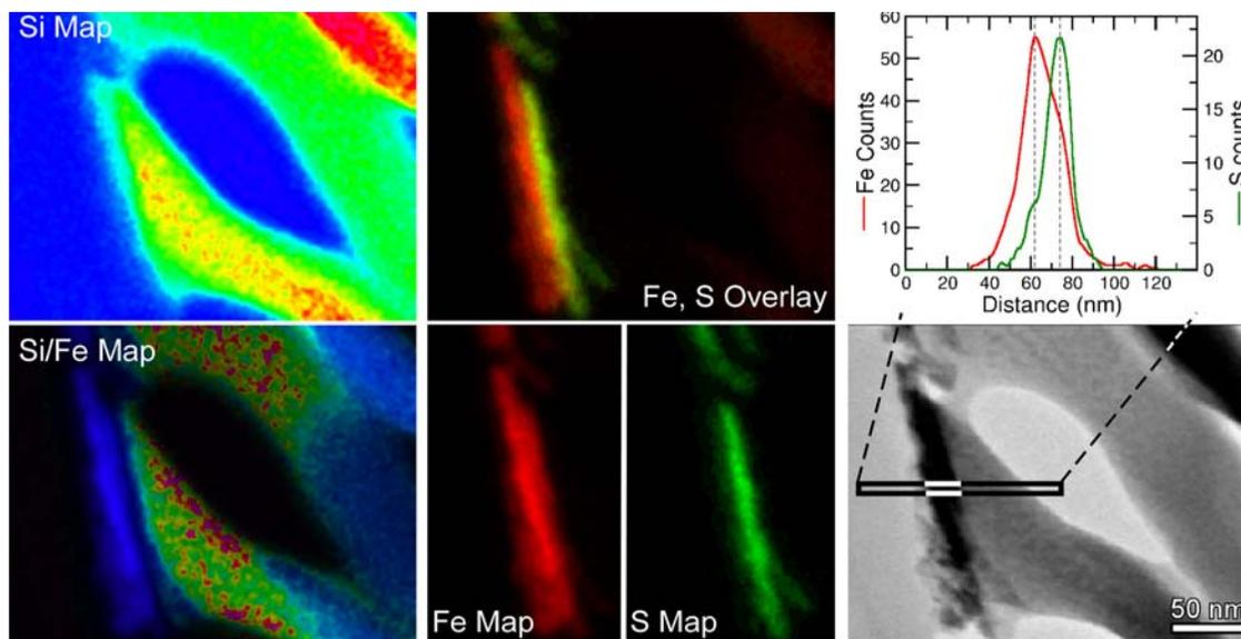
**Figure 2:** FESTEM/EDS X-ray map of surface deposits on cross-section of Apollo 15 volcanic green glass bead.
