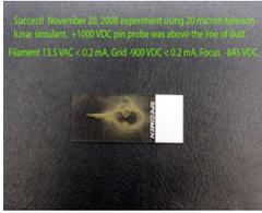
Figure 5. Successful induced dust migration with a focused electron beam in the presence of an electric field.
