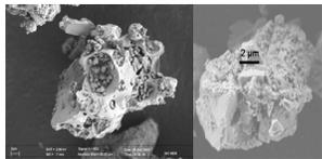
Figure 1: SEM photo of grains comparing surface morphology of Lunar Dust (left) and simulant (right) illustrating size distribution, clumping, and complexity of smaller particles
