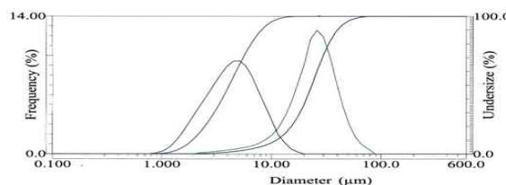
Figure 4 Normalized frequency and cumulative frequency distributions for lunar simulant at t=0 (right) and at t=60 seconds (left) when only the finest fraction remains in solution. Note the presence of an ultra fine component at or below 3 microns.
