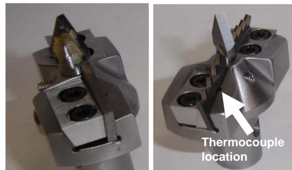
Figure 2: Drill bits used for drill study.
