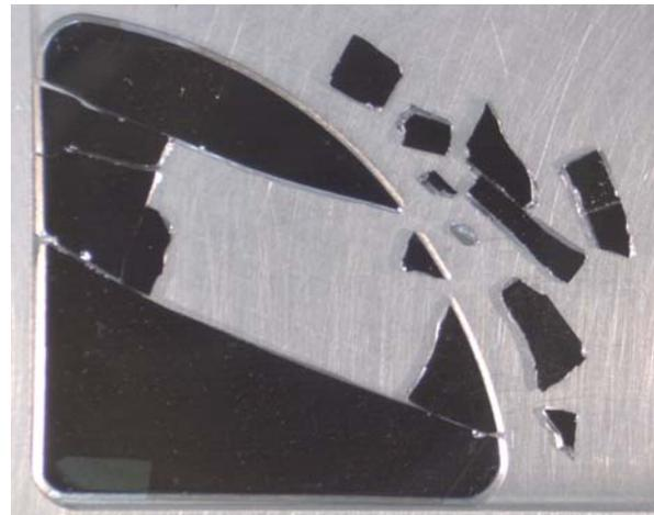
Fig. 3. DLC-on-silicon quadrant fragments fitted together, ambient illumination, Leica MZ9 microscope.
