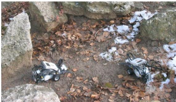
Fig. 2. Field works between rocks at early winter. Leaves form special obstacles for the small rovers.
