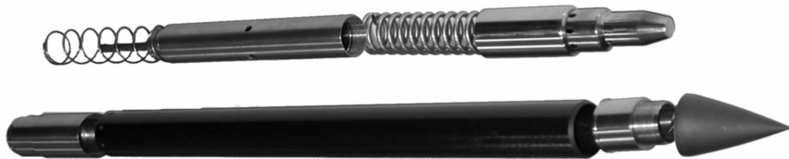
Fig 1. The laboratory model of the mole penetrator: the outer tube with the tip (bottom) and the hammer with the countermass (top).
