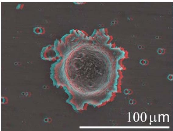
Figure 3. SEI stereo anaglyph of a large bowl-shaped crater, produced by a fine-grained olivine aggregate.
