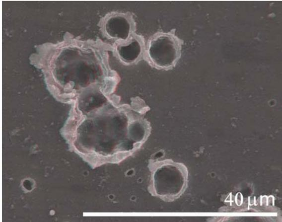
Figure 2. Secondary electron image (SEI) stereo anaglyph of complex crater made by fine olivine aggregate experimental impact on Stardust foil.
