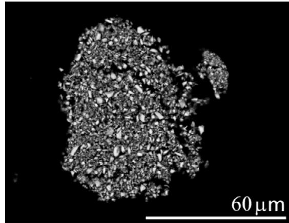
Figure 1. Backscattered electron image of a cross section through an artificial olivine aggregate projectile.
