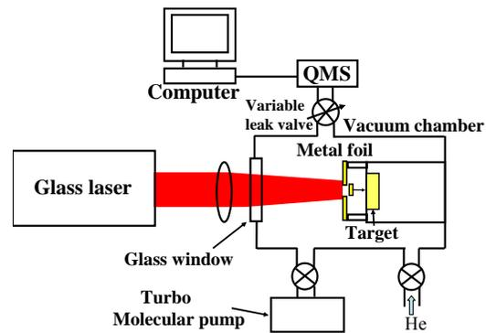
**Figure 1.** A schematic diagram of our experimental system. It consists of a Glass laser, a vacuum chamber, a turbo molecular pump and a quadrupole mass spectrometer (QMS).
