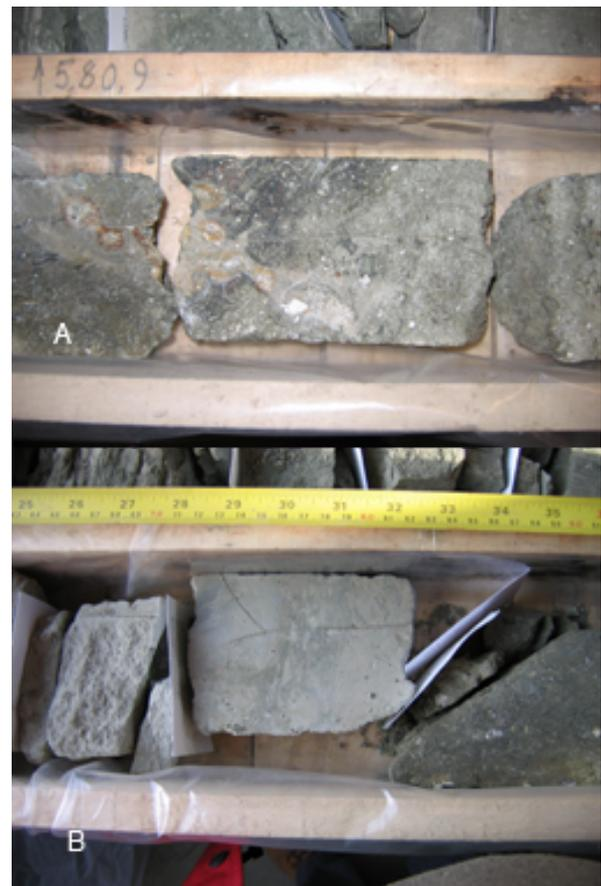
**Figure 1.** Images of core material recovered from the Boltysch impact crater. (a) Suevite breccia from a core depth of 580.9m and (b) Contact between suevite breccia and overlying lacustrine sediments at 581.5m.
