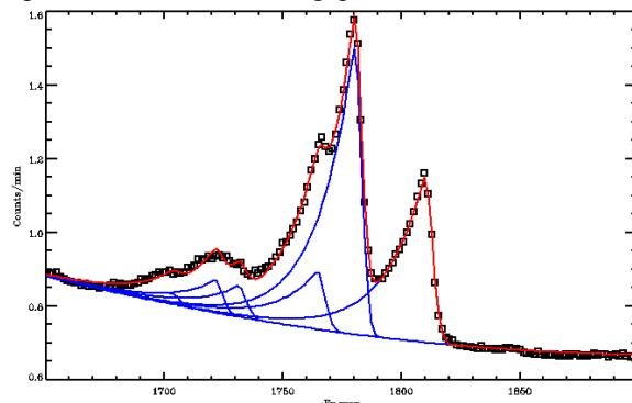
Fig. 2 Example of a peak fitting result of the  $^{238}\text{U}$  peak in an energy spectrum observed by the SELENE GRS. Black dots represent the actual observed count rate in each energy bin, the blue lines represent individual peak components, and the red line represents the total fitting result.
