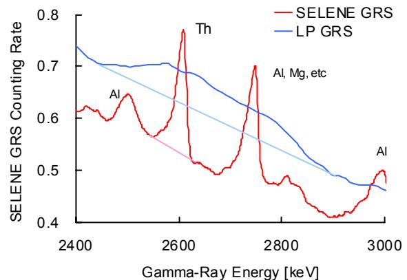
Fig. 1 Comparison of the Th gamma-ray peak at 2615 keV observed by the SELENE GRS and that by the LP GRS [10,11]. The SELENE GRS uniquely resolved individual peaks, contributing precise assessment of elemental abundances. The vertical axis for the LP GRS spectrum is arbitrary.
