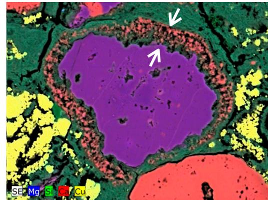
**Fig. 4.** Combined BSE image and EDS element map for a dolomite clast with Si-Al-Ca-rich phyllosilicate corona (between arrows) from the uppermost 0.5 mm of the spherule deposit in ODP Site 1259B.
