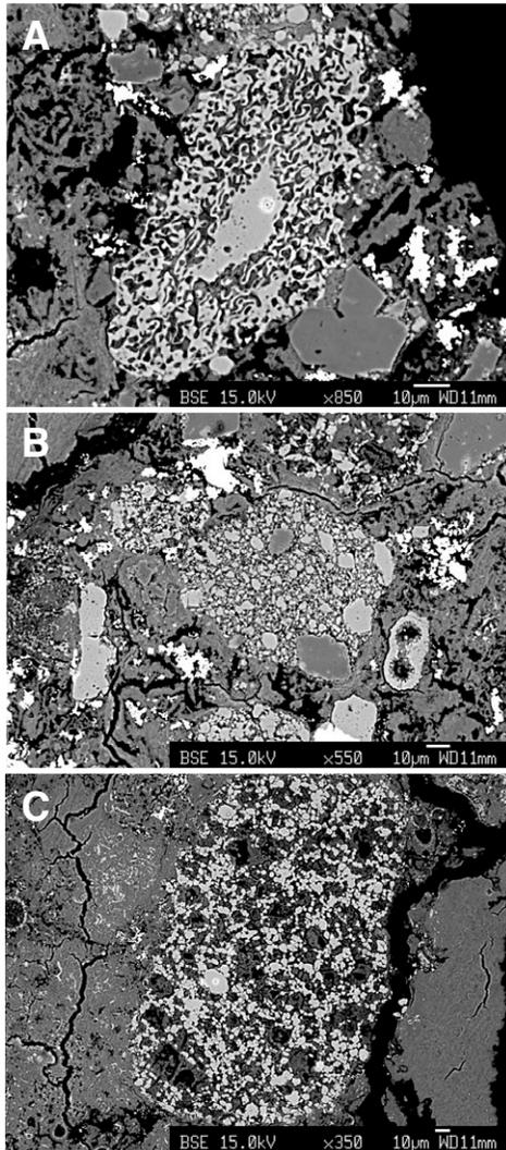
**Fig. 3.** BSE images of carbonate clasts in the uppermost 0.5 mm of the spherule deposit in ODP Site 1259B. (A) Rounded porous calcite clast, note distinct flow-shaped pores; (B) carbonate clast consisting of accreted  $\mu\text{m}$ -sized calcite and dolomite sub-grains; (C) highly porous accretionary calcite clast composed of  $\mu\text{m}$ -sized calcite sub-grains and (dark gray) smectite matrix.
