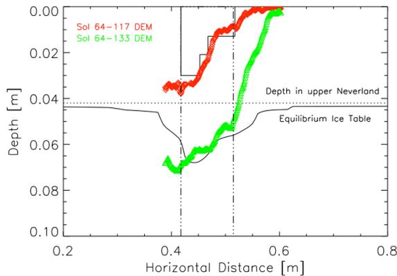
Fig. 3. Transects of DEMs approximating (red) the shape of Headless below the soil and (green) the underlying ice table and entrance ramp of the Pet Donkey trench. Vertical dashed lines indicate the horizontal extent of Headless visible at the soil surface. Solid lines represent an irregular rock and the corresponding ice table predicted by ice-stability simulations. Horizontal distance increases radially outward from the spacecraft.
