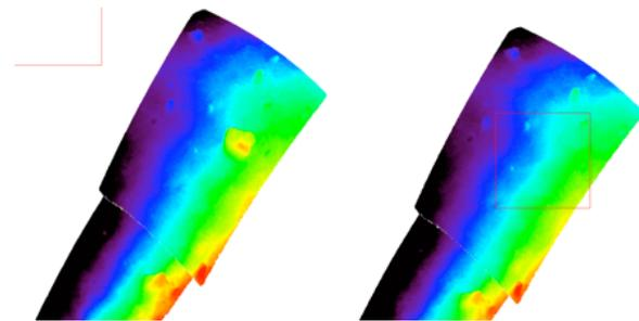
Fig. 2. Original “pre-dig” DEM (left), and modified DEM with Headless removed by interpolation (right).
