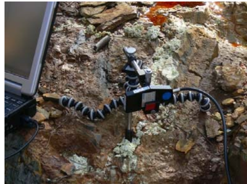
Figure 1. Raman optical head taking spectra on the mineral precipitates at the Rio Tinto source
