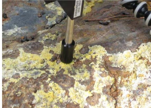
**Figure 1:** Raman probe working in-situ on a mineral efflorescence.
