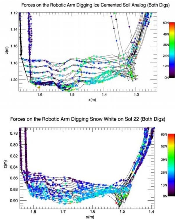
Figure 5. Curves of depth vs. horizontal distance. Data points are color-coded by force. (above) Laboratory tests with ice cemented soil analog. (below) Snow White from the first sol it was dug into. Snow White was the most frequented trench of the mission.
