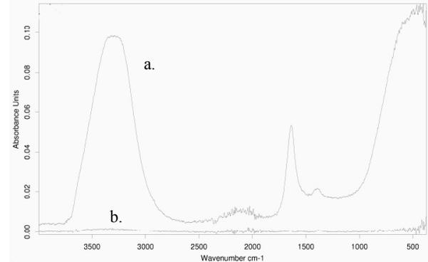
**Figure 1.** IR spectra for NWA 869. a) pH 12.95 for 5 months. b) pH 7 for 3 months.
