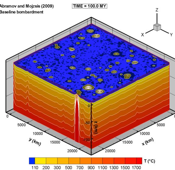
**Figure 1.** A 3-dimensional model representing the Earth’s lithosphere at the end of the 100 Myr LHB. Only impactors larger than 10 km in diameter are included in this model. Dark areas denote crater imprints.
