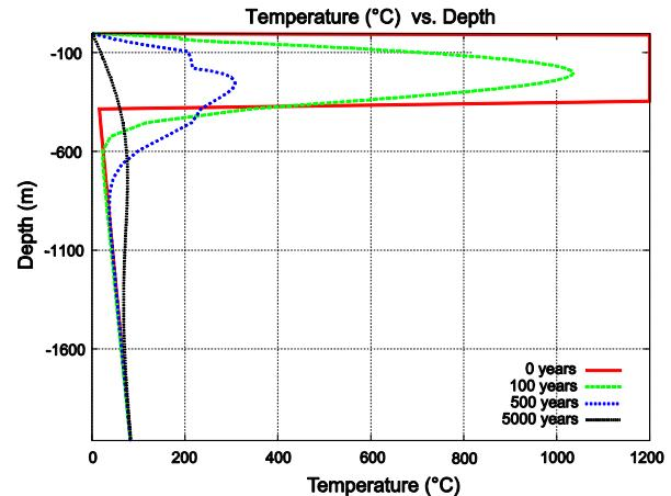
**Figure 3.** Cooling of a 350 m thick, 1200 °C global ejecta blanket as modeled using the computer code HYDROTHERM. Cooling by hydrothermal venting is included.
