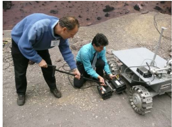
Fig. 2: ExoGeoLab Test of Electromagnetic interference of a Ground Penetrating radar with a mid-size rover platform
