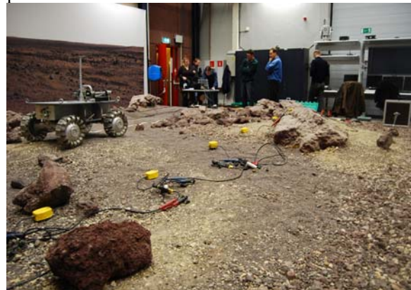
Fig. 1: ExoGeoLab tests of a Geophone system and Ground Penetrating Radar at ESTEC Planetary Robotics Testbed
