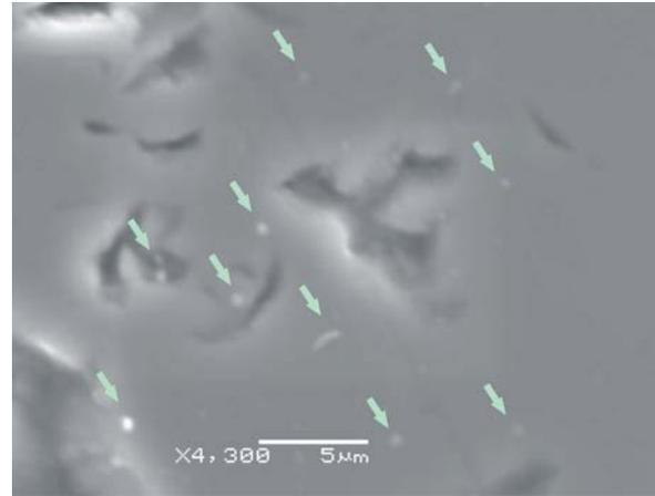
Figure 1. SEM images of the np-Fe<sup>0</sup> in the glass phase by microwave heated (hold 8 minutes). The arrows point to the np-Fe<sup>0</sup>.
