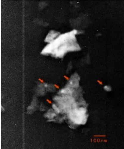
Figure 2. TEM images of the np-Fe<sup>0</sup> on the silicate minerals surfaces of the CLRS-2 by magnetron sputtered. The arrows point to the np-Fe<sup>0</sup>.
