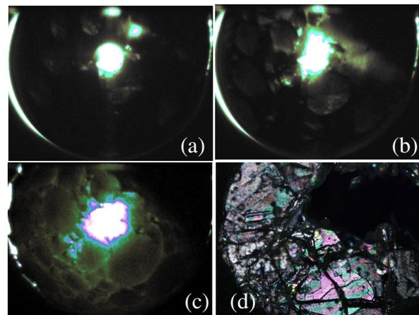
Figure 2: (a-c) Time sequence of instantaneous shadowgraph images showing the transient evolution of the crystallization process inside the silicate melt droplet; (d) Photomicrograph of thin section of the silicate spherule showing the porphyritic texture at the end of the crystallization process.
