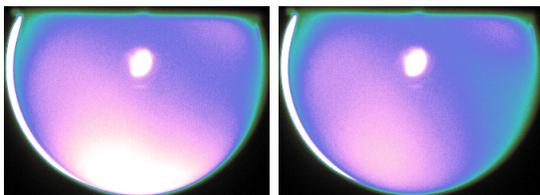
Figure 1: Sequence of schlieren images (false color) showing the transient evolution of melt convection inside the silicate melt droplet.
