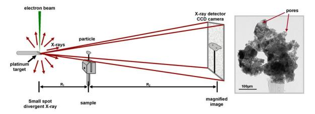
Fig.1 Schematic diagram of an X-ray ultramicroscope showing a 2-D projection image of an agglutinate particle.
