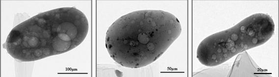
Fig.3 X-ray ultramicrographs of opaque glassy particles with ellipsoid, teardrop and dumb-bell morphologies.
