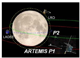
**Figure 1:** ARTEMIS will study with two identical, cross-calibrated spacecraft lunar exospheric ions and dust, crustal magnetism, and the lunar interior. One probe will measure the pristine solar wind driver, while the other will study the lunar environment's response. ARTEMIS extends the SELENE/Kaguya results into the next decade, providing synergy with LRO, LADEE, and the International Lunar Network.
