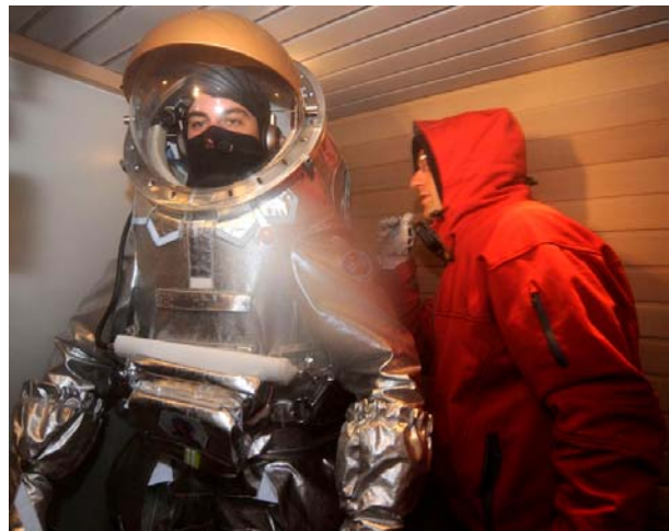
Fig. 1: Aouda.X spacesuit simulator at cryotests at -110°C prior to the Eifel field campaign
