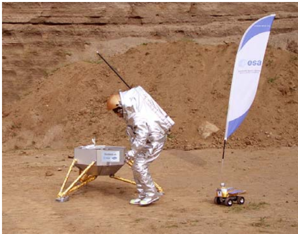
Fig. 2: The ExoGeoLab lander simulator is being inspected by the crew explorer in Aouda.X EVA suit
