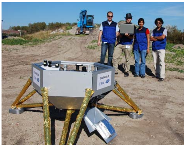
Fig. 2: ESTEC test of ExoGeoLab lander with remote operations of door and instruments
