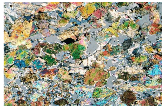
Figure 3. (above) Plane polarized light image; olivine (brown), clinopyroxene (beige), plagioclase (white), Fe oxides and shock glass (black). (below) Partially cross-polarized light image. Widths 9 mm © T. Bunch.
