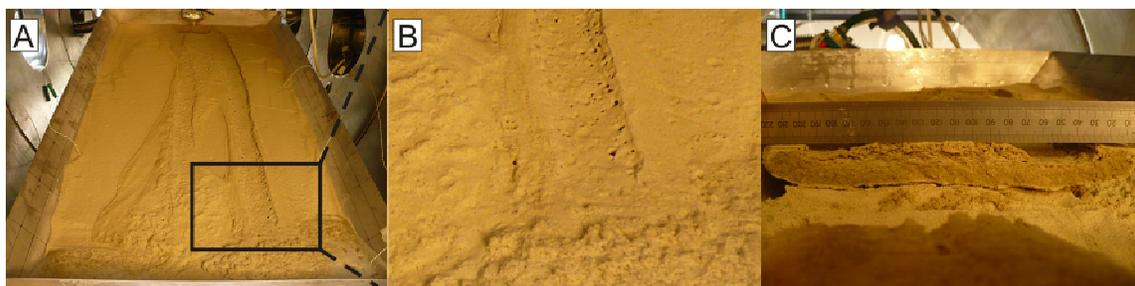
**Figure 1.** Photos after experiment 090619\_001 with fine sand: (A) the whole sediment tray, (B) zoom-in on inset marked in (A), showing lateral levees, bubbles in the channel and rough texture of icy deposits, and (C) cross section of the flow near the top, showing the ice-lens, clear channels and lots of bubbles throughout the upper 1 cm.
