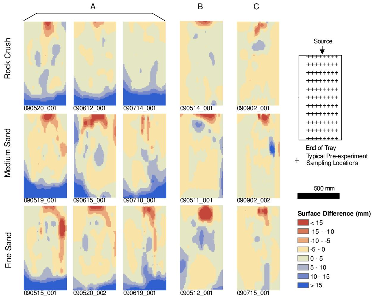
**Figure 2.** Matrix of isopach maps for each experiment. Each row is a different sediment type and each column represents different ambient experimental conditions, with **A** being low temperature/low pressure, **B** ambient temperature/low pressure and **C** ambient temperature/ambient pressure. Diagram top right shows typical arrangement of measured points pre-experiment. After the experiment, more measurements were taken around areas of greatest change.
