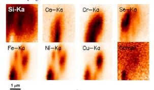
Fig. 3: X-ray fluorescence and Compton map of I1043,1,30.
