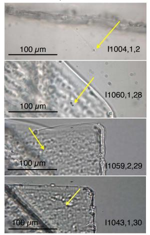
Fig. 2: Optical images of tracks I1004,1,2; I1060,1,28; I1059,2,29; I1043,1,30. Arrows point to terminal particles.
