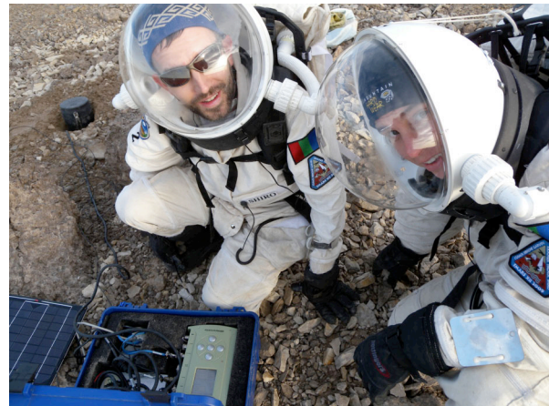
Figure 1: Brian Shiro and Christy Garvin test the seismometer (upper left) before burying it.
