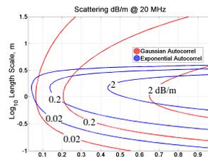
**Figure 3.** Born scattering at 20 MHz for two different autocorrelation functions. Meter-scale heterogeneity with  $\sim 30\%$  velocity variations ( $\sim 40\%$  differences in dielectric constant) yields attenuation
