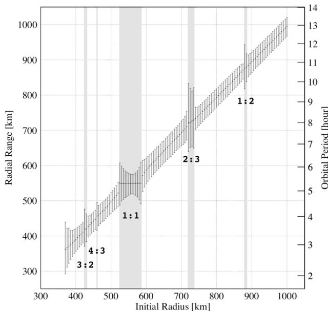
**Figure 2.** Dynamics of the Dawn spacecraft spiraling in from HAMO under 20 mN thrust, becoming trapped in the 1:1 resonance between Dawn's orbital period and Vesta's rotational period. Trapping is sensitive to the equatorial longitude at which Dawn crosses the resonance.
