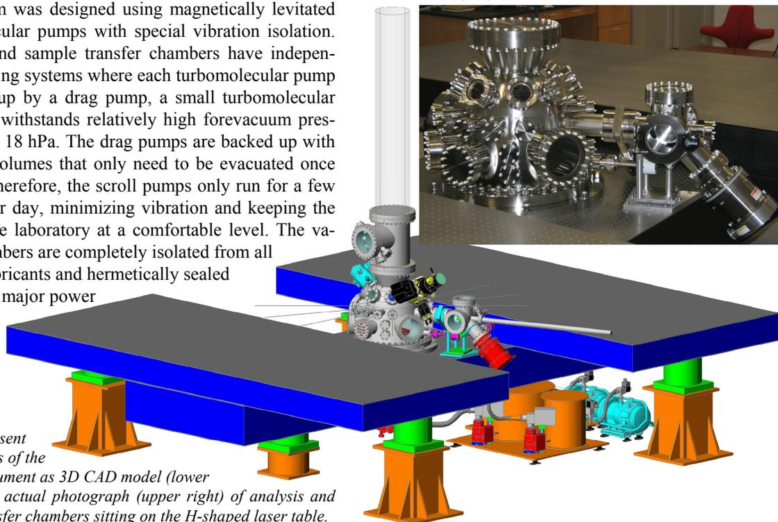
Figure. Present design status of the CHILI instrument as 3D CAD model (lower left) and an actual photograph (upper right) of analysis and sample transfer chambers sitting on the H-shaped laser table.
