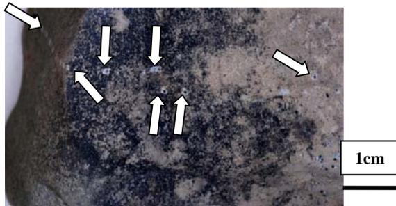
**Fig. 4** TLH-1, a massive carbonate showing epilithic/endolithic colonization. LIBS laser pits shown by arrows.
