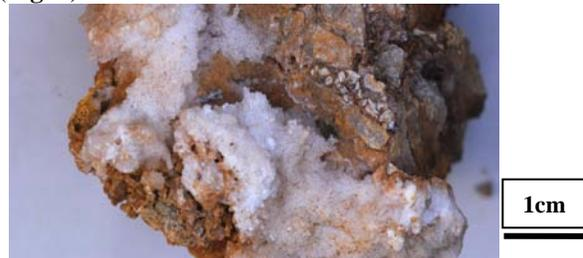
**Fig. 2.** TLH-9, impact breccia of carbonate clasts cemented with iron oxides and coated with a white precipitate mineral.
