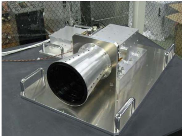
**Figure 1 : Test model of the LIR onboard Akatsuki**
