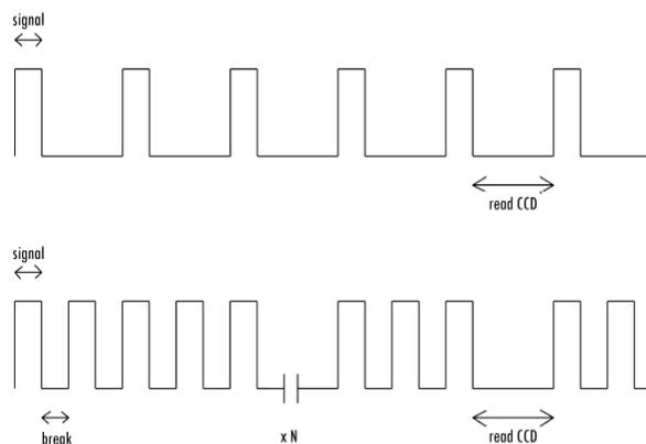
Figure 1 Modification of basic CCD readout method to mimic electronic shutter system.
