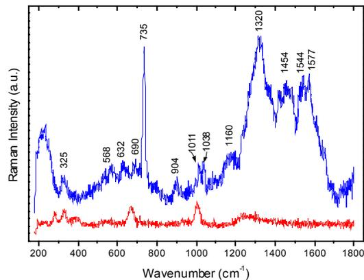
Fig 3. Raman spectra of adenine adsorbed on DAG 670 pyroxene before (red line) and after (blu line) the addition of silver nanoparticles.
