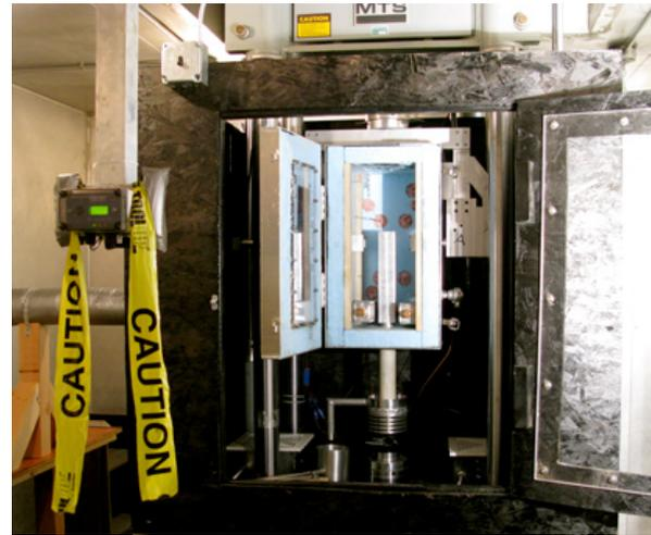
Fig. 2. Photograph of testing system in a cold room showing MTS model 810 uniaxial loading frame and normal/side loading device, box for containing nitrogen gas and oxygen sensor suspended from ceiling.
