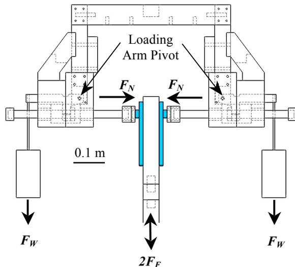
Fig. 1. Engineering drawing of double shear device.
