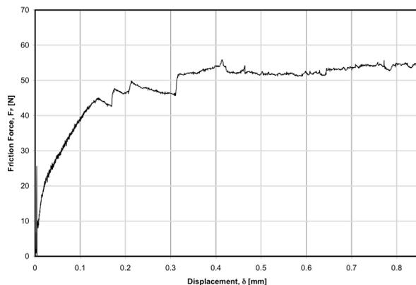
Fig. 3. Typical  $F_F$  vs.  $\delta$  curve.  $V=5\times 10^{-8}$  m s $^{-1}$ ,  $F_N=130$  N, granular ice ( $d=8$  mm).
