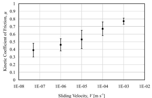
Fig. 4. Kinetic coefficient of friction vs. sliding velocity of ice on ice at  $-175$  °C.
