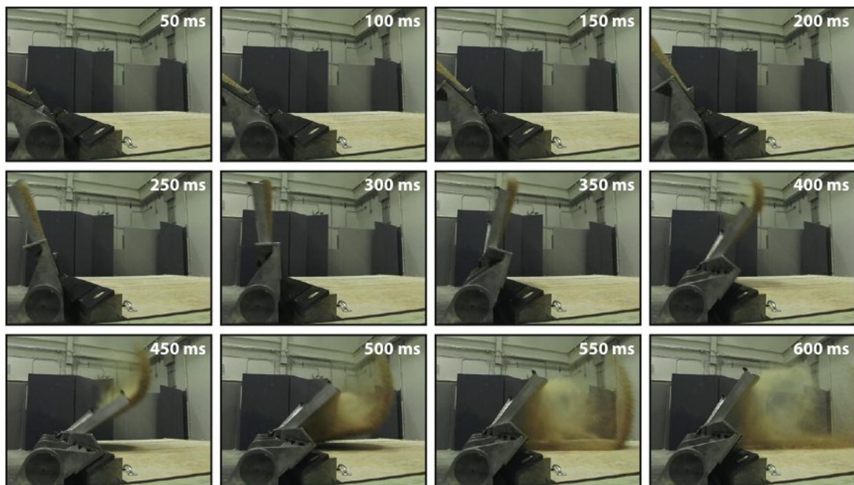
**Figure 3.** Data from the first EESim experiment showing ejection and emplacement of debris analogous to ejecta. The time elapsed since release of launcher plate is indicated in each frame.
