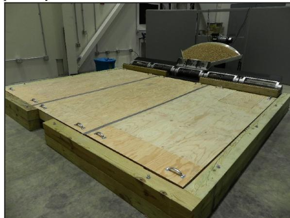
**Figure 2.** The front of the EESim with its ejecta launcher plate loaded.
