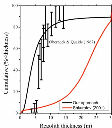
**Figure 2.** Cumulative distribution of regolith thickness for the region in Figure 1. The black line represents the results from this study, the red line is from Shkuratov and Bondarenko [5], and the data with associated error bars are from the crater morphological investigations of Oberbeck and Quaide [4].
