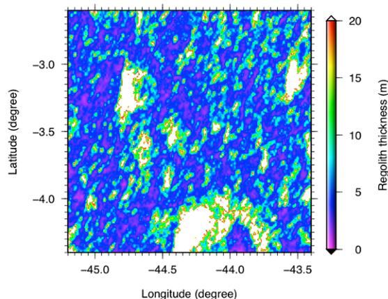
**Figure 1.** Inverted regolith thickness for a region close to the Surveyor 1 landing site (site 9.2b in [4]). The average regolith thickness at this site was estimated to be 8-9 from crater morphology study [4].
