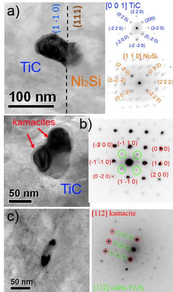
Fig.2. a) BF image and microdiffraction patterns of TiC with  $\text{Ni}_2\text{Si}$  attached to its (1 -1 0) face. b) BF image of TiC with 2 attached kamacites and diffraction pattern from upper kamacite with extra  $\text{Fe}_2\text{Si}$  spots c) BF image of FeSi-rich phase consisting of 3 crystalline domains and diffraction pattern from lower domain.
