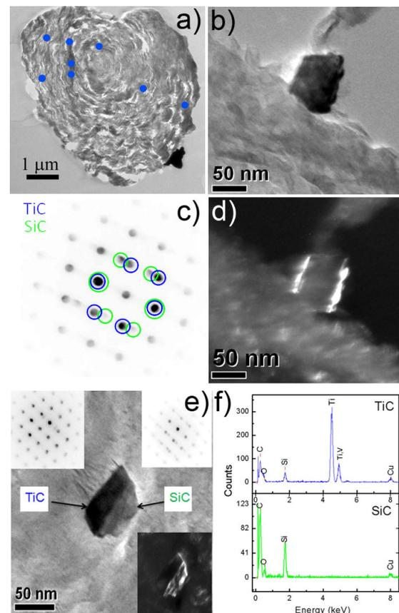
*Fig. 1. a) Bright-field (BF) image of g18 graphite with internal TiCs indicated by blue dots b) bright-field image of TiC and c) microdiffraction pattern taken from edge of 1b showing SiC coating phase grown onto TiC face. d) DF image from SiC spot revealing SiC coatings (bright) on opposite (111) TiC faces e) BF and DF images of TiC/SiC composite grain including diffraction patterns and f) EDXS from each side.*
