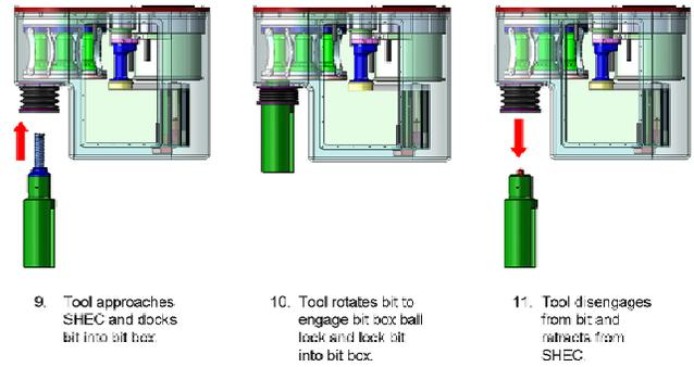
Figure 7. Manual bit transfer from tool to SHEC.
