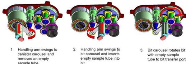
Figure 4. Automated tube insertion in SHEC.
