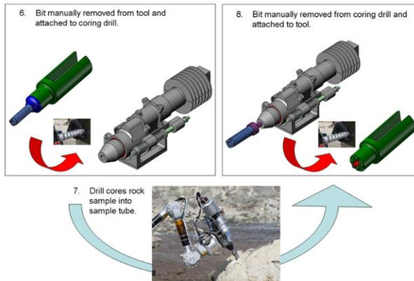
Figure 6. Manual bit changeout and coring.
