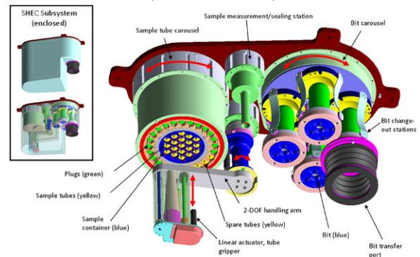
Figure 2. The Sample Handling, Encapsulation, Containerization subsystem (SHEC).
