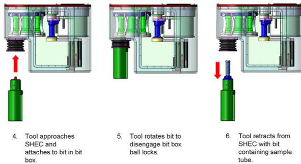
Figure 5. Manual bit transfer from SHEC to tool.
