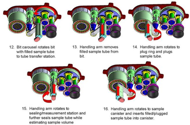
Figure 8. Automated tube sealing in SHEC.
