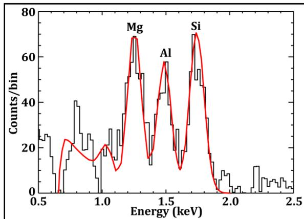
Figure 2: Background subtracted, C1XS spectrum (0.5 - 2.5 keV) for ROI 13 of the observation (see Fig. 1). The characteristic Mg, Al and Si  $K_{\alpha}$  lines are well resolved (no higher energy lines are excited during this low-magnitude flare). The modelled fit (red line) is generated using a solar flare model at a temperature of 3.1 MK. The lines below  $\sim 1.0$  keV are due to scattered solar X-rays rather than XRF.
