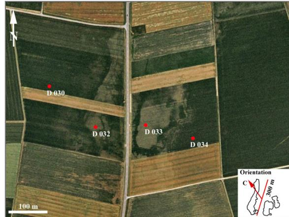
**Fig. 1:** Google Earth image of a crystalline megablock structure near Alerheim. Points indicate the location of the corresponding drilling sites. D032 and D033 yielded weathered crystalline material at a depth of ~30 cm. D030 and D034 did not reveal evidence for crystalline material in the borehole profiles down to ~3 m depth. The arrow in the megablock sketch indicates the direction of the crater center.
