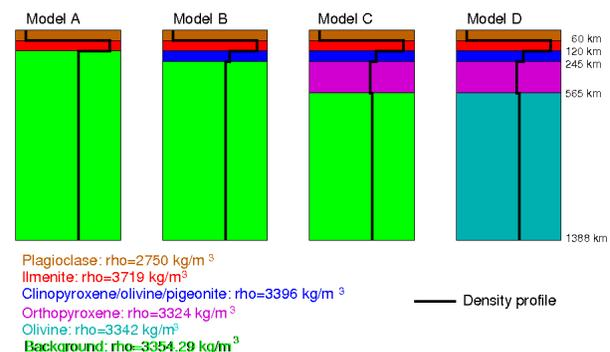
Figure 2: Initial setup of the models with different numbers of layers
