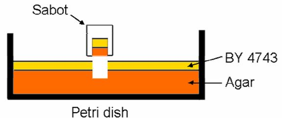
**Fig. 1** Schematic showing loading of a sabot with yeast spores via a 'cookie cutter' method.
