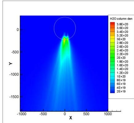
**Figure 4:** Water column density, as viewed from Saturn, of South Polar plumes as simulated by free-molecular model with DSMC initialization (axis values are in km). The white circle represents Enceladus.
