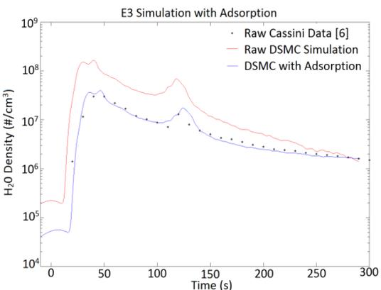
**Figure 6:** E3 simulation accounting for adsorption in the INMS antechamber by convolution with assumed instrument function.
