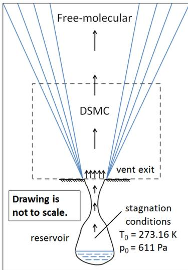
**Figure 1:** A schematic of the simulation regimes. DSMC is used in the collisional flow near the vent while the free-molecular model is used further out where the flow is mostly collision-less. The reservoir conditions are assumed to be the triple-point of water.
