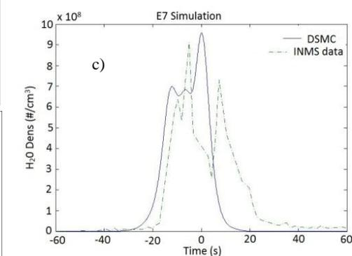
**Figure 5a, 5b, and 5c:** Comparison of *in situ* INMS data [6] and raw simulation results for a) E3 flyby, b) E5 flyby, and c) E7 flyby utilizing DSMC particle initialization.
