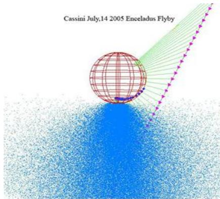
**Figure 3:** Visualization of Cassini E5 flyby through free-molecular south polar plumes of Enceladus. The green lines and red arrows indicate the spacecraft trajectory, while the blue squares represent the spacecraft groundtrack.
