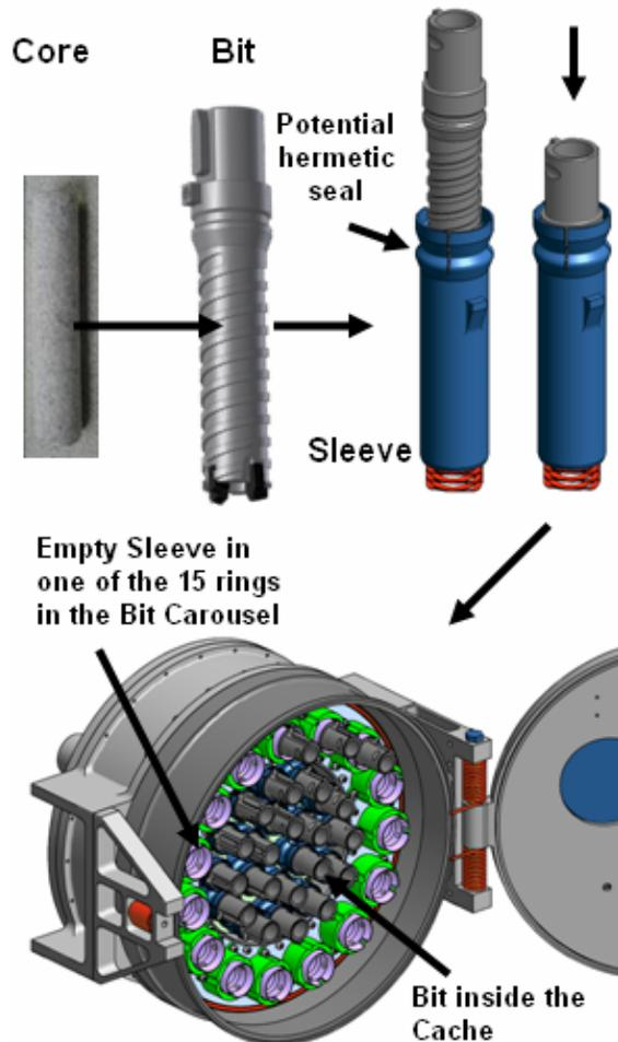
**Figure 2.** Cores are stored inside individual bits. The bits with cores inside them are inserted into dedicated sleeves within either the Cache or the Bit Carousel (for temporary storage). The bits with sleeves can be pulled out of the Bit Carousel and inserted into the Cache.
