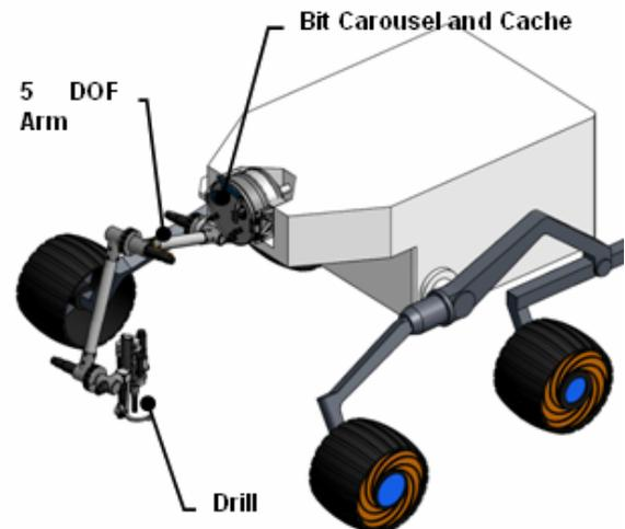
**Figure 1. Sample Acquisition and Caching system in its deployed position.**
