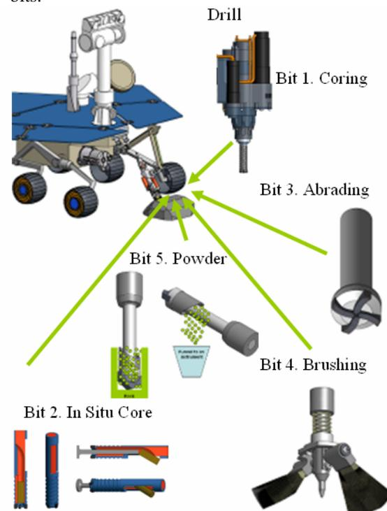
**Figure 3.** The drill can be used with 5 different bit types for in-situ rock interrogation.
